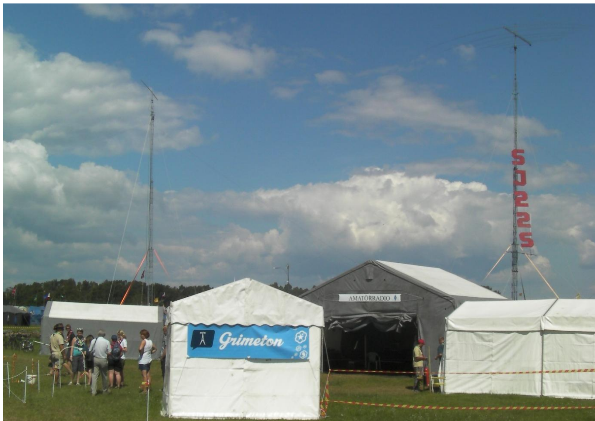
The 2 M beam is on the left tower. The logperiodic is above the callsign. The 3 el beam isn't visible here
